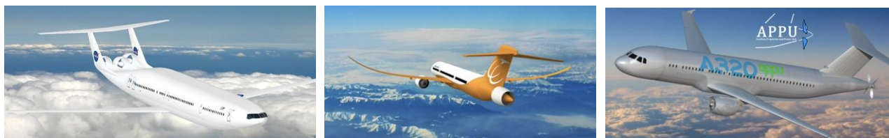
Figure 20: Examples of novel aircraft concepts that utilize boundary layer ingestion (BLI), a) MIT D08 design (MIT, 2010; Drela, 2010; NASA, 2010), b) Propulsive fuselage concept (CENTRELINE, 2017), c) TU Delft APPU project (TU Delft, 2020)
