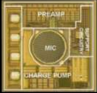
Monolithic CMOS MEMS Microphone Chip
