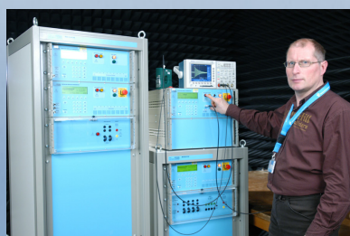
Test equipment for lightning induced susceptibility tests
