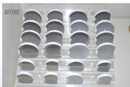
Salt spray test for the replacement of chroming plating as applied on landing gears (left side before the test, right side after 192 test hours)
