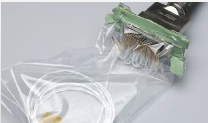
▲ Proved seal methods for connectores and test cables
